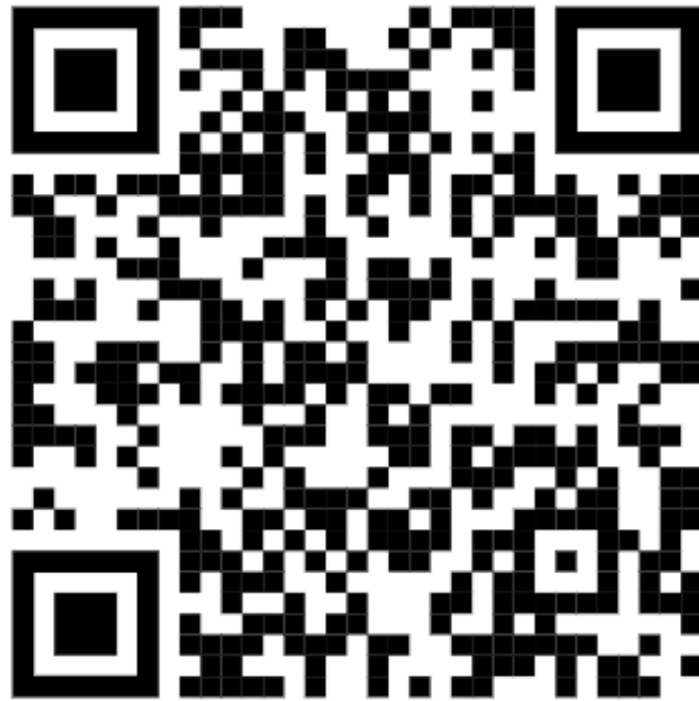
Figure 2 – QR code in the form of a Reed-Solomon code with 4 redundant characters, containing the text “Test object No. 1”
