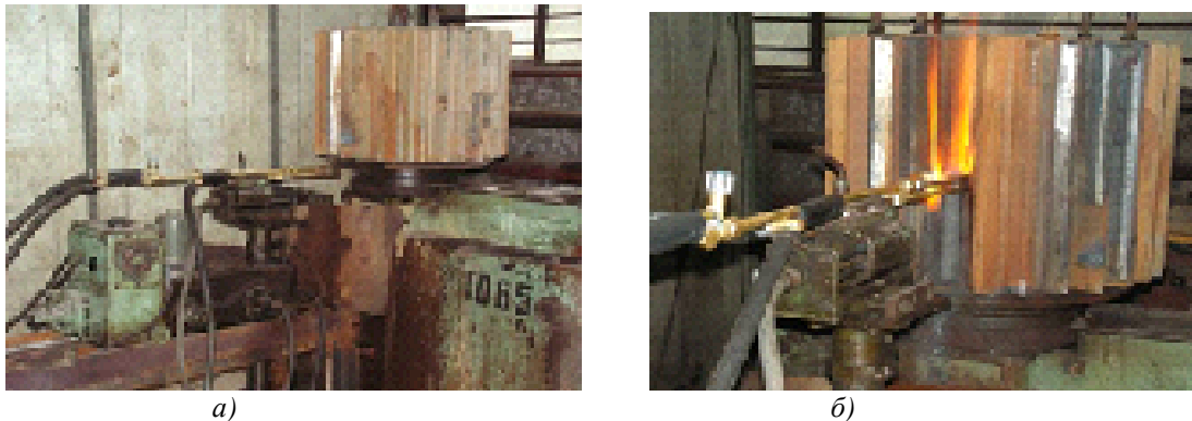
Fig. 1 – Worn large gear wheels: a) a worn cylindrical gear wheel; б) a worn cylindrical gear wheel surfacing
